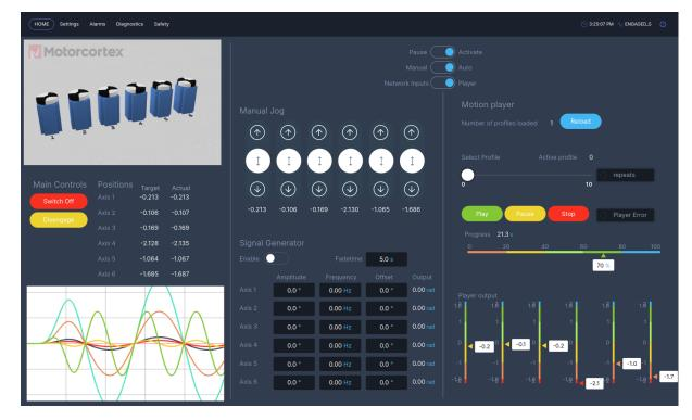
Motorcortex-Machine-App is a turn-key motion control software for a general class of Machines. The Machine-App provides the machine logic, motion control, errorhandling and interfacing to hardware. Shorten your time-to-market and reduce software development
